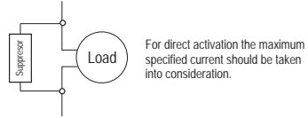
Diagram for suppresor installation for direct drive load inputs
